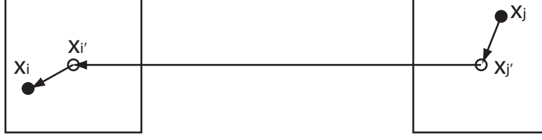
Figure 1: Decomposition of distance vectors into three parts
